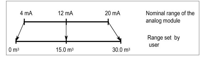
The Scaling Values (SCALE) function takes an integervalue (IN) and converts it to a real value in engineering units scaled between a low and a high limit (LO\_LIM and HI\_LIM). The result is written to OUT.
